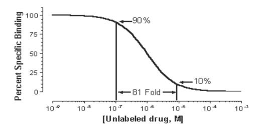
The steepness of the curve is the "Hill slope" which should be ~ -1
